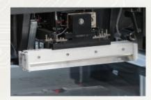
New quick release squeegee blades makes changing blades quick and easy with no tools required. It takes less than 30 seconds to change the blade.
