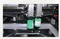
Dispense for standard cartridges or choose the new patent-pending jar dispenser. Paste is released in precise, measured amounts across the stencil in a
