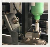
Temperature monitoring ensures proper paste viscosity to avoid bridging and voiding. MPM patent-pending paste temperature monitor allows paste to be measured in the cartridge or on the stencil.
